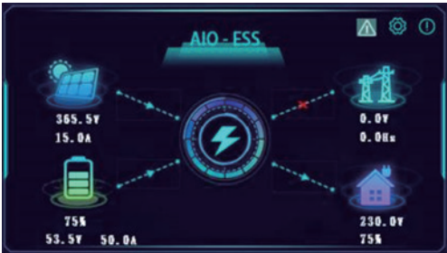
▲ Batteries and solar power supply the load .
